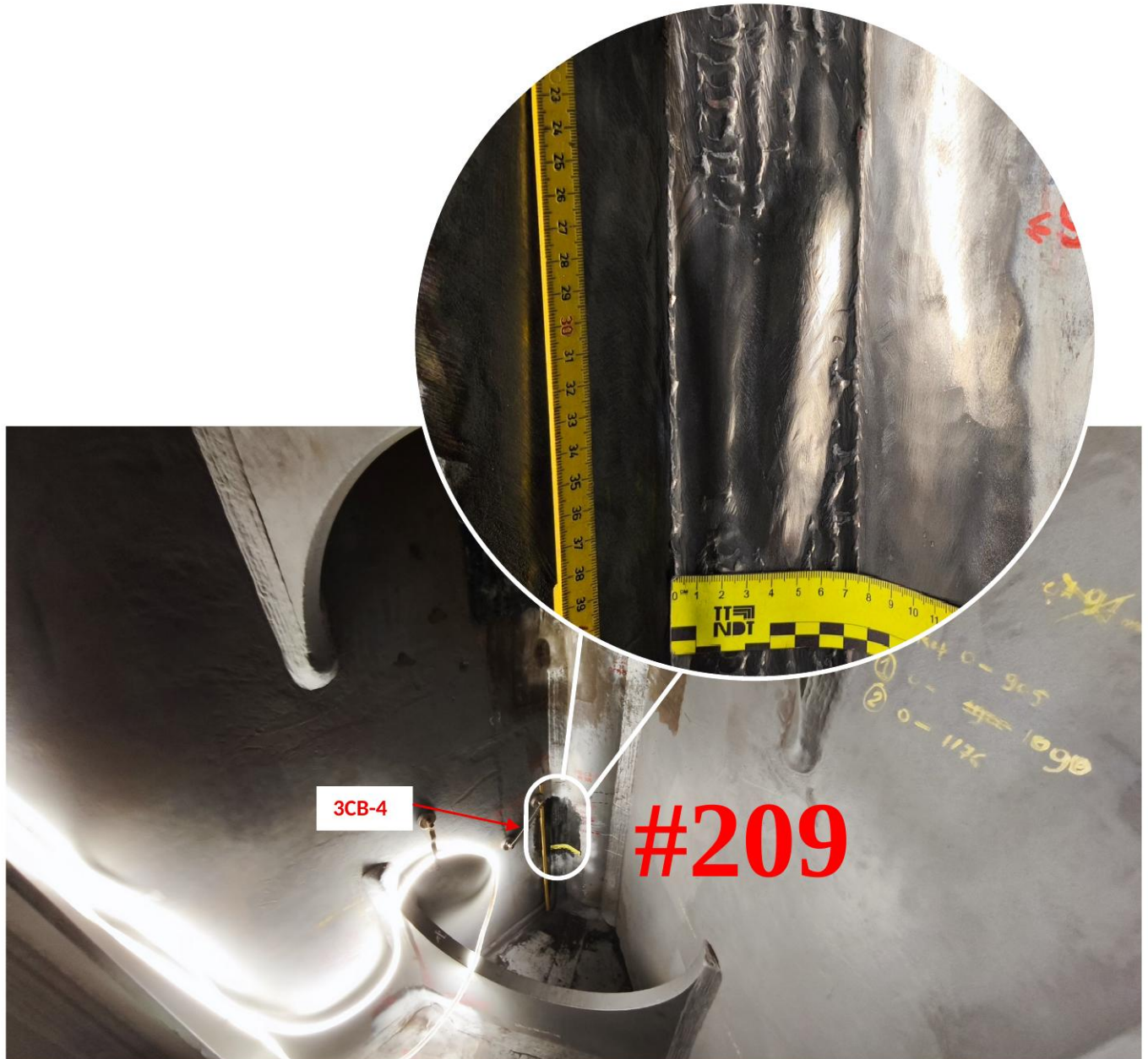
Picture 1: Spud Can 3, Chord C, Noble indication No. 206, Force Indication No. 3CB-4, Weld No. S3I-CB-SP overview
